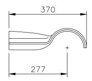
CEMBRIT LIMITED CEMSIX TWO-PIECE CLOSE VENTILATION RIDGE OUTER (LEFT) NET COVER: 1016mm Drg. No.330
